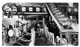
DETROIT - It began on Oct. 7, 1913, when engineers constructed a crude system using a rope and winch to pull a Ford Model T past 140 workers in a sprawling new factory dubbed the Crystal Palace.
