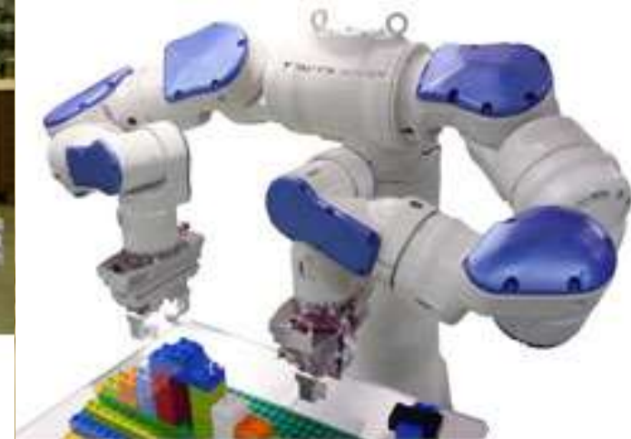
A dual-arm, 15-axis collaborative robot with human-like flexibility in a small footprint (Courtesy of Yaskawa Motoman Robotics, Miamisburg, Ohio)
