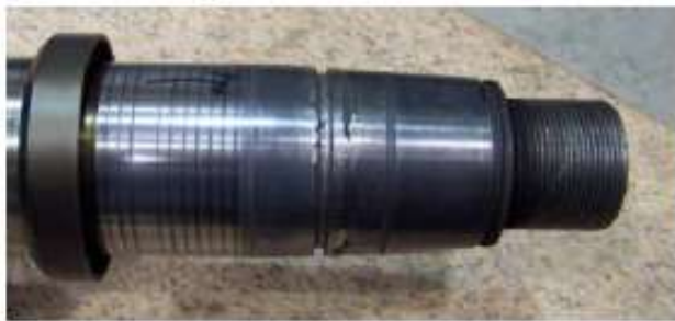
Atomizer Shaft as Received
