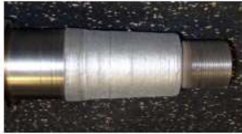
Atomizer Shaft with Laser Deposit
