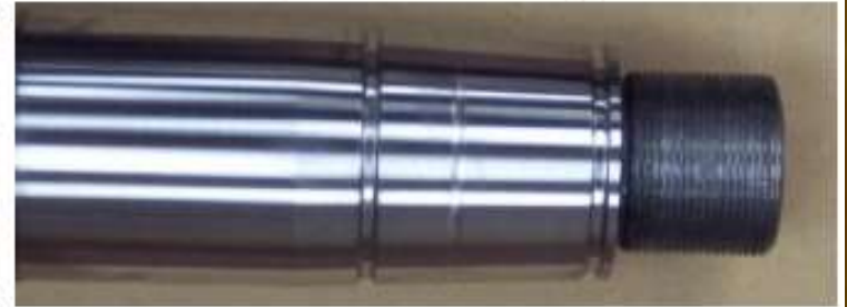
Atomizer Shaft Final Machining
