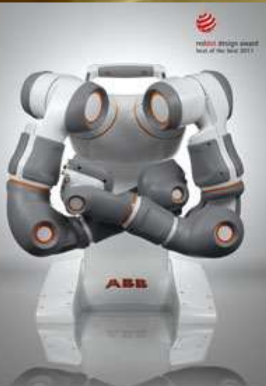
Dual-arm concept robot for collaborative small-part assembly operations (Courtesy of ABB Inc.)
