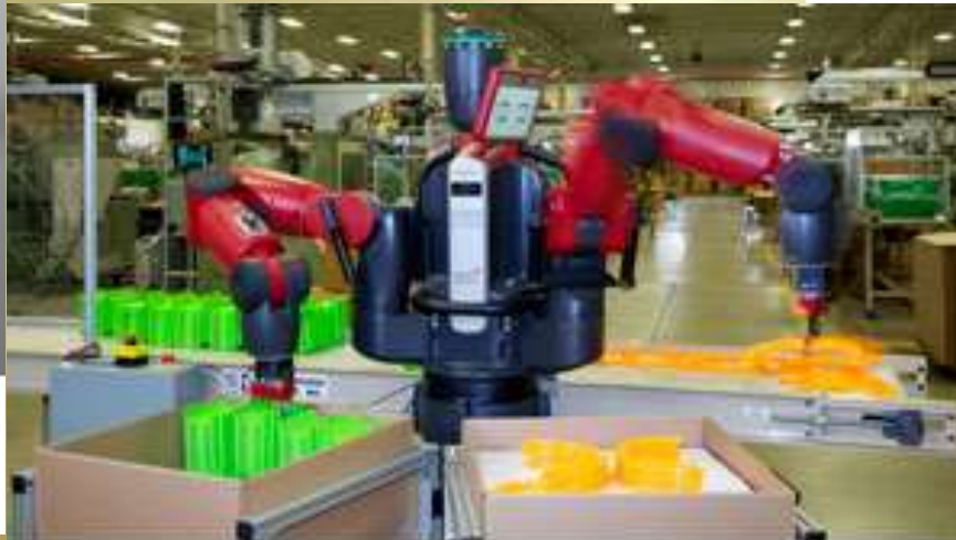
Baxter, a dual-arm collaborative robot, packs plastic parts into boxes on the factory floor (Courtesy of Rethink Robotics, Boston, Massachusetts)
