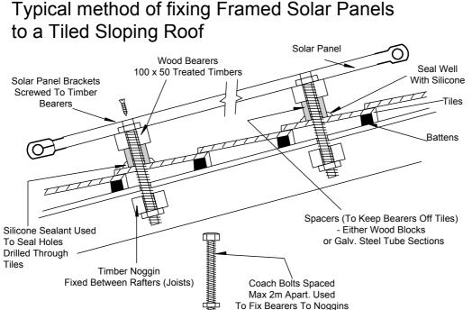
Mounting the framed panels (Models 030 and 020) on the roof is relatively simple since the two bearers must be at the same distance apart as the top and bottom fixing brackets on the panels.
