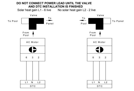
When it is necessary to plumb the outlet pipes to pool and panels into opposite valve ports reverse L1 and L2 as follows:
