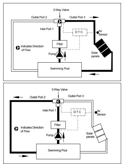
The inlet from the pool must always be on the branch port (1) of the valve. The outlet ports (2 & 3) can be as shown in diagram above or reversed as detailed overleaf.
