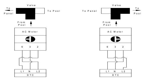
Solar heat gain L1 - 2 live No solar heat gain L2 - 6 live
