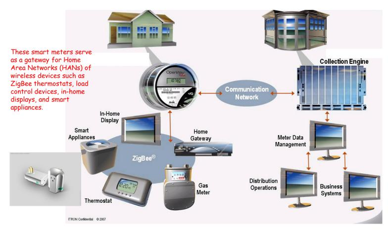
**ZigBee** is a specification for a suite of high level communication protocols using small, low-power digital radios based on the IEEE 802.15.4-2003 standard for Low-Rate Wireless Personal Area Networks (LR-WPANs), such as wireless light switches with lamps, electrical meters with in-home-displays, consumer electronics equipment via short-range radio.
