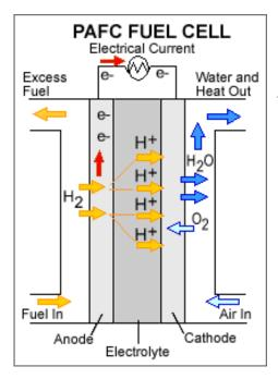
Phosphoric acid fuel cells use liquid phosphoric acid  $(H_3PO_4)$  as an electrolyte—the acid is contained in a Teflon-bonded silicon carbide matrix and porous carbon electrodes containing a platinum catalyst.
