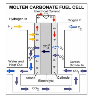
MCFCs are high-temperature fuel cells that use an electrolyte composed of a molten carbonate salt mixture suspended in a porous, chemically inert ceramic lithium aluminum oxide (LiAlO<sub>2</sub>) matrix. Because they operate at extremely high temperatures of 650°C (roughly 1,200°F) and above, nonprecious metals can be used as catalysts at the anode and cathode, reducing costs.
