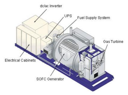
Since the SOFC stack operates at 1000°C it produces a high temperature exhaust gas. If operated at an elevated pressure, the exhaust becomes a hot pressurized gas flow that can be used to drive a turbine.
