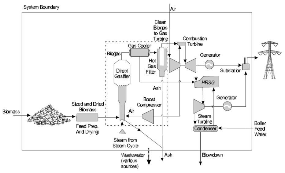
Biomass gasification combined cycle (BGCC) system schematic.
