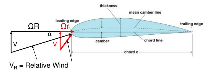
$\alpha$  = angle of attack = angle between the chord line and the direction of the relative wind,  $V_R$  .
