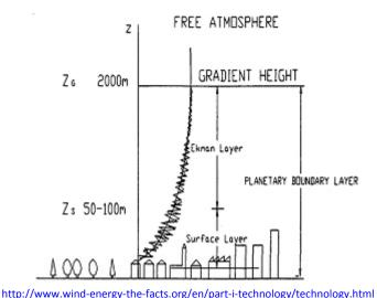
*Surface roughness* determines to a certain extent the amount of turbulence production, the surface stress and the shape of the wind profile.
