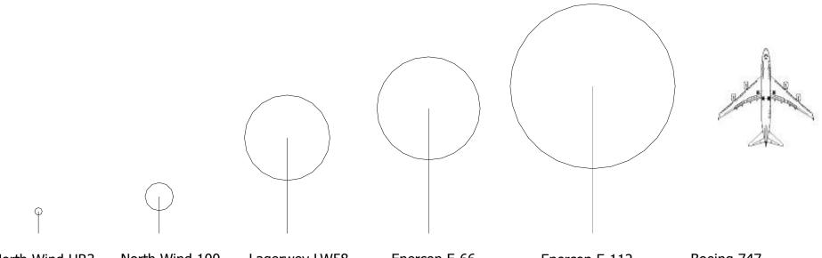
North Wind HR3North Wind 100rating: 3 kWrating 100 kWrotor: 5 mrotor: 19.1 mhub height: 15 mhub height: 25 m
