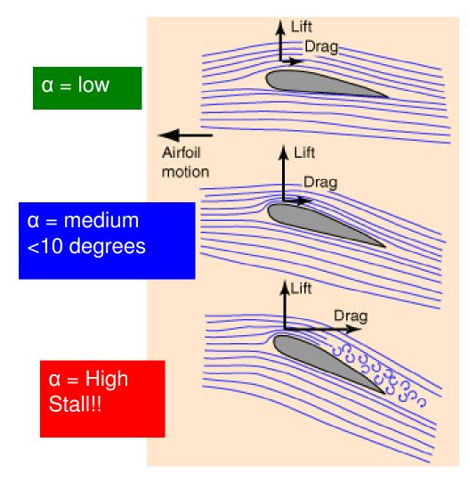
The <u>Drag Force</u> is parallel to the direction of motion. We want to make this force small.
