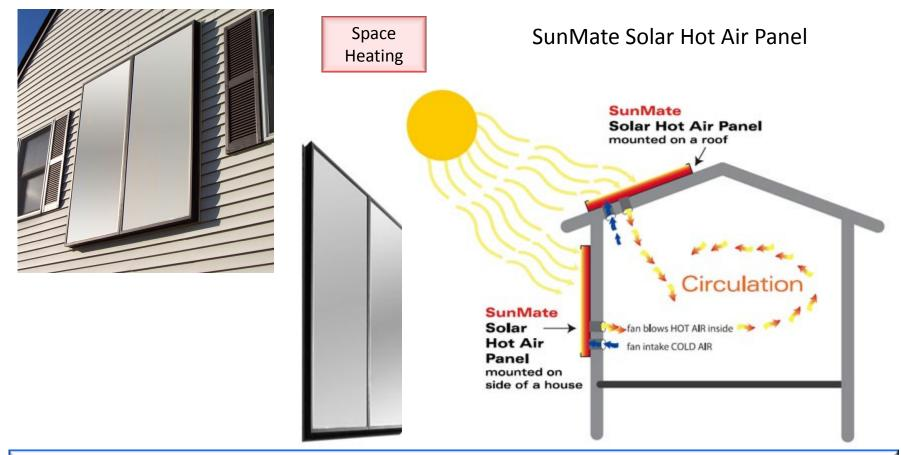
Pulls cool air from your home, channels it through the absorber plate where it's warmed by energy from the sun, then circulates it back into your home. A built-in thermostat, automatically turns on a blower when the absorber plate reaches 110° F and shuts off the blower at 90°F.
