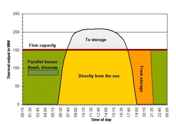
Typical output of a solar thermal power plant with two-hour thermal storage and backup heating system to guarantee capacity.
