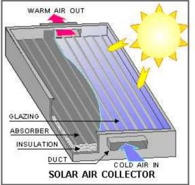
Air based systems begin producing heat earlier and lasts longer during the day than liquid bases systems of approximately the same size. Consequently, ventilation, heating and preheating is possible earlier. Besides heating individual spaces, heated air can also heat air passing into air recovery ventilators or air converters of heat pump systems.
