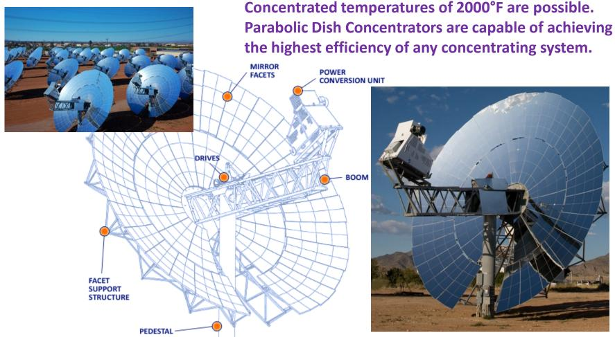
The SunCatcher<sup>™</sup> is a 25-kilowatt-electrical (kWe) solar dish Stirling system which consists of a radial solar concentrator dish structure that supports an array of curved glass mirror facets, designed to automatically track the sun, collect and focus solar energy onto a Power Conversion Unit (PCU). The PCU is coupled with, and powered by, a **Stirling engine that generates** electricity.
