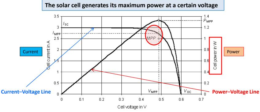
This graph shows the current-voltage and power-voltage characteristics.
