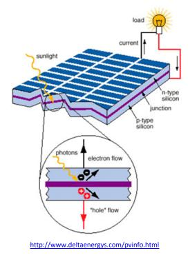
Simplified schematic of solar cell operation.
