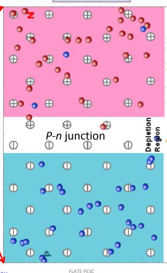
On the *n*-type side, positive ion cores are exposed
