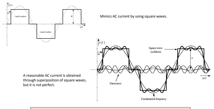
DC to AC Inverters modify DC signals, which are constant, to AC signals, which as we have seen vary in a sinusoidal pattern.
