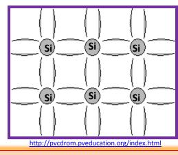
Schematic of covalent bonds in a Silicon crystal lattice
