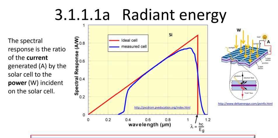
The spectral response of a silicon solar cell under glass. At short wavelengths below 400 nm the glass absorbs most of the light and the cell response is very low. At intermediate wavelengths the cell approaches the ideal. At long wavelengths the response fall back to zero.
