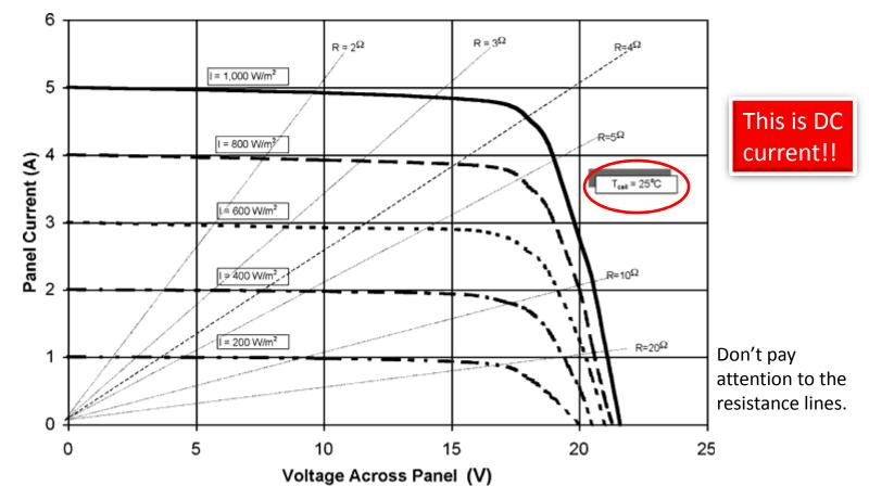
A single silicon photovoltaic cell produces an open-circuit voltage of slightly over 0.55 volts. The voltage produced by a photovoltaic panel is a function of how many cells are connected in series. In the case of the panel described above, there must be about 36 photovoltaic cells
