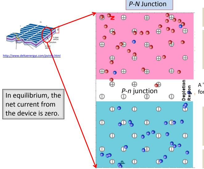
On the *n*-type side, positive ion cores are exposed
