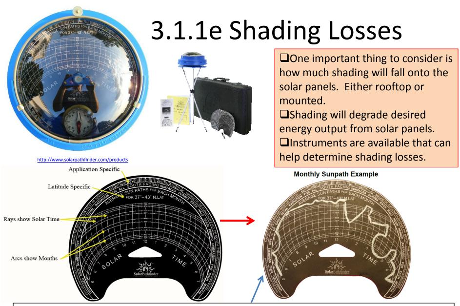
To find the site percent, add the numbers in the unshaded part of the sunpath arc. The site tracing shown here has 64% solar available for January, found by adding 2 + 3 + 4 + 5 + 6 + 7 + 7 + 8 + 8 + 6 = 64%. This shows that only 64% of the potential available radiation is reaching this particular location during January. 36% of the potential available radiation is blocked out in the middle of the winter.
