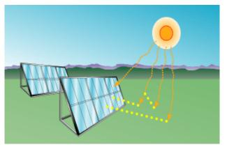
Flat-plate collectors, which typically contain a large number of solar cells mounted on a rigid, flat surface, can make use of both direct sunlight and the diffuse sunlight reflected from clouds, the ground, and nearby objects. ✓ The global irradiance on a horizontal surface on Earth consists of the direct irradiance  $E_{dir}$  and diffuse irradiance  $E_{dif}$ .
