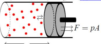
When heat is added, the molecules gain kinetic energy, which in turn causes more bouncing and more force on the piston.
