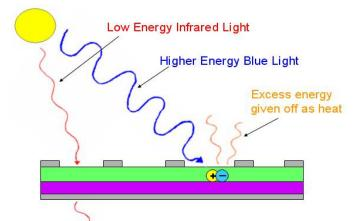
As mentioned before, sunlight is made of light with a broad range of energies spanning from infrared to ultraviolet light. Low-energy light doesn't have the energy required to release electrons; too-high energy light wastes the excess energy as heat.
