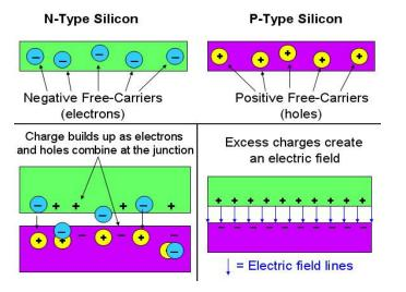
N-type silicon has negative freecarriers (electrons), while P-type silicon has positive free-carriers (holes). When the two materials are put together, a junction is formed. At this PN Junction, electrons are attracted to holes and move to the P-type silicon via a conductor.
