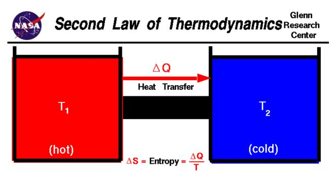
There exists a useful thermodynamic variable called entropy (S). A natural process that starts in one equilibrium state and ends in another will go in the direction that causes the entropy of the system plus the environment to increase for an irreversible process and to remain constant for a reversible process.
