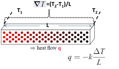
$$(1.4 \text{ W/mK})(20 \text{ K/0.2 m}) = 140 \text{ W/m}^2$$
