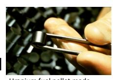
Uranium fuel pellet made from compaction of Uranium Dioxide powder. Not in enriched form here.
