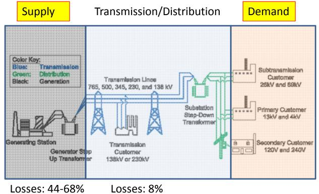
•Under current electricity distribution design , electrical energy is not typically stored.
