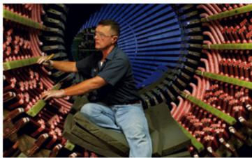
stator of a 225-megawatt air-cooled electrical generator to be used in a combined cycle power plant.
