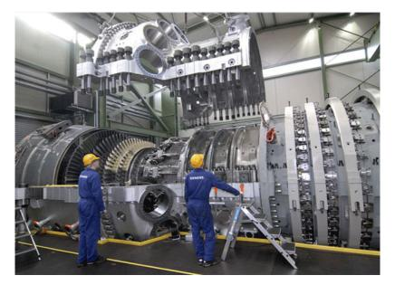
Siemens SGT-8000H series gas turbine designed to achieve more than  $_{FLATE-FES}$  60% efficiency in combined cycle operation. 375MW stand-alone
