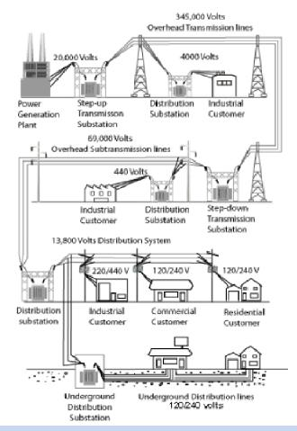
AC transmission lines carry three-phase current and use three transmission lines. DC transmission uses two lines- one for positive current and one for negative current.
