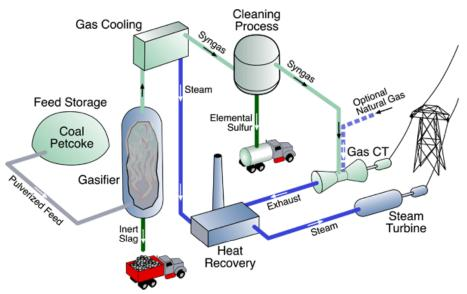
Integrated Gasification Combined Cycle (IGCC) plant
