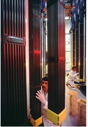
Reactor Fuel Assembly: Pellets are stacked within each rod. Several rods make up the assembly.
