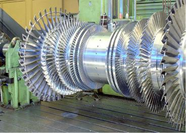
The SST-500 is a single casing, double flow steam turbine with up to 100 MW power output.
