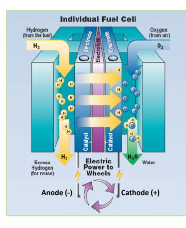
$2H_2 + O_2 \rightarrow 2H_2O + Electrical power + heat$
