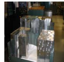
Figure 7. Aluminum Blocks used to build valves
